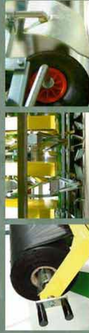
Support rollers / Plastic roller support - Distributore a tazze / Cup distributing system - Gruppo ribottezza film / Film covering system
