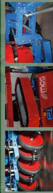
Ruote costipatrici / Treading wheels
